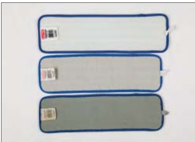
18" Wet Pad backing discoloration.
