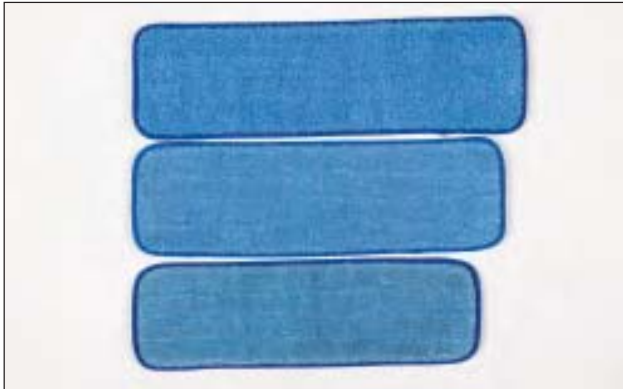
18" Wet Pad shrinkage due to high heat.
