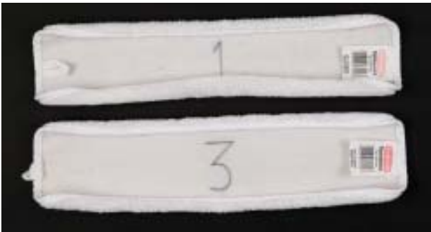
18" Room Dusting Pads curling up due to high heat.
